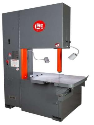
**6V-36 BAND SAW** Speed indicator, six speed gear box, 3:1 variable speed drive, speed range 20-15,000 F.P.M., automatic wheel brake, door limit switches, 5/8" - 1" 3 piece guides and holders, two work lights, 15 H.P. 208/230/460 volt, 3 phase, 60 cycle, 1725 R.P.M. TEFCBB brake motor, NEMA 12 enclosure.
